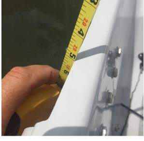
squarely in the middle of the mast partners when pulled forward snug against the shrouds. To ensure similar mast bend from side to side when sailing, a centered mast in the partners is more important than a mast centered in the boat side to side. Ideally the mast would be centered in the partners as well as being even side to side but sometimes things just aren't equal.....
